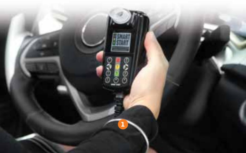
If you qualify to participate in the program, an ignition interlock device will be installed in your vehicle. The device is designed to stop a vehicle from starting or operating when the driver has been drinking.
