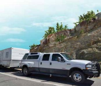
When attached, your towing vehicle and trailer can be **up to** 21.5 m (70 ft) long. When apart, each can be **up to** 12.5 m (41 ft) long.
