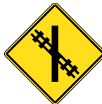
Railway crossing advance warning, track position indicates the angle the railway tracks cross the road
